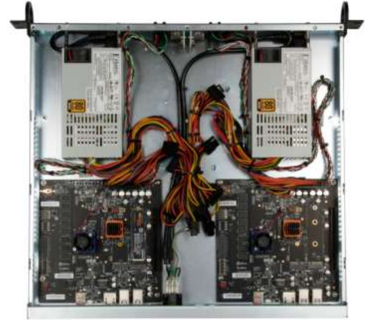
Experimental university sample: 2 (of 6) HiFive Unmatched boards, SiFive Freedom U740 SoC, 16GB of 64-bit DDR memory, gigabit Ethernet, Infiniband Host Channel Adapter (HCA, 56GB/s, RDMA). Couldn't run the SW stack
